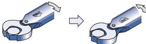
Use by turning over the torque wrench
