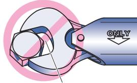
In case that you do not insert the nut to the full depth of SP, accurate tightening torque is not applied due to change the effective length and it causes damage of spanner.
