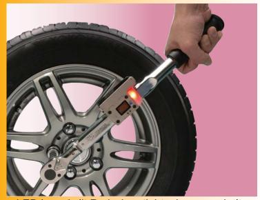
LED lamp is lit Red when tightening same bolt which already tightened with required torque.
