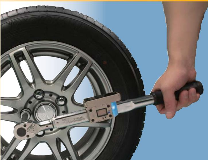
Completion of tightening process with Blue signal
