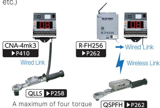
A maximum of four torque wrenches can be connected to the count checker. In case of wireless, I/O-FH256 is required.
