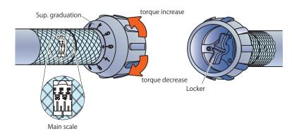
Loosen locker, and twist sup. graduation Tighter locker once torque setting completed.
