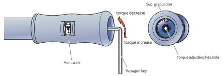
Insert the hexagon key into the torque adjusting hex, hole and turn the hexagon key to set the torque.
