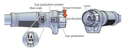
Loosen locker, and twist sup. graduation Tighter locker once torque setting completed.
