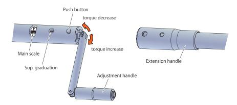
Push the Push button and remove the extension handle. Turn adjustment handle built in the wrench to set the torque. Finally, attach the extension handle.
