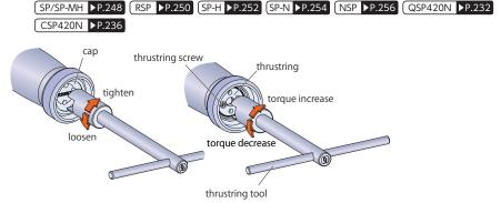
Remove the cap using thrustring tool. Loosen the thrustring screw and turn the thrustring. Torque wrench tester is needed for comfirming the torque value.
