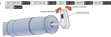
Insert the adjusting tool and turn it.
